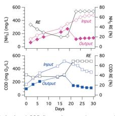
Fig. 7 NH<sub>3</sub> (top) and COD (bottom) averaged concentrations before (input) and after (output) an electrochemical treatment cycle of 4 hours with respective removal efficiencies (RE) for 30 continuous days of operation of YXG prototype. Day 0 corresponds to the beginning of usage of the prototype.
