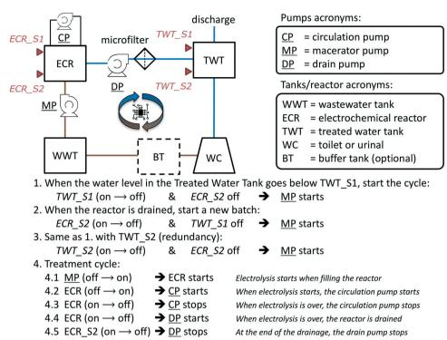
Fig. 3 System flow diagram (top left, see Fig. S1† for volumes and residence times) with automation algorithm description for the onsite toilet wastewater treatment and recycling systems. Pumps are underlined. Capacitive level sensors are represented by red triangles. Brown lines illustrate the flow of untreated wastewater while blue lines illustrate the flow of treated and recycled wastewater.
