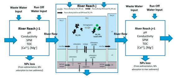
Fig. 5 Schematic representation of the ENP transport into, out of and throughout the defined river reaches and fate processes inside the river system. Adapted from Praetorius et al. 2012.<sup>52</sup>
