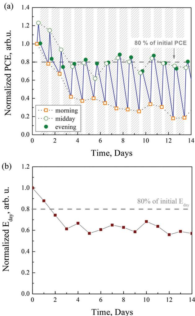
Fig. 2 (a) PCE evolution of type II mini-modules (glass/ITO/TiO<sub>2</sub>/MAPbI<sub>3</sub>/Spiro-OMeTAD/Au) during their outdoor sunlight exposure. (b) Evolution of the daily energy output generated by this cell. For simplicity, we used a constant  $P_{\text{in}} = 1 \text{ Sun}$  for the  $E_{\text{day}}$  calculation. All lines are guides for the eye.
