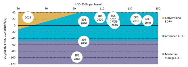
Fig. 21 Sensitivity of economic viability and choice of CO<sub>2</sub>-CCS-EOR approach to oil and CO<sub>2</sub> prices, reproduced from IEA.<sup>968</sup> The circles indicate different ETP future scenarios: e.g. 2DS 2030 indicates where a 2 °C capped mean global temperature rise world may be positioned in 2030.
