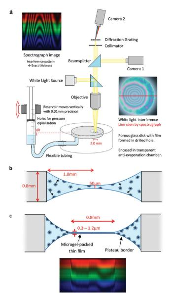
Fig. 1 (a) Experimental set-up used to study the drainage of thin-liquid films made from microgel suspensions. (b) Time t = 0 s. Microgels shown schematically; actual diameter 700 nm. The interfaces are 50 µm apart at the closest point and do not interact. Time allows for microgels to diffuse and adsorb to the interface. (c) Shape of the film after hydrostatic pressure is applied and drainage begins. The interferometry spectrum for a typical film is also shown.
