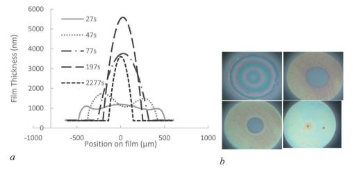
Fig. 3 (a) Drainage dynamics and thickness profile for the 1.5 mol% BIS microgels at 0.1% wt as a function of time. (b) White light images of the thin-liquid foam films as a function of time for 18, 80, 500 and 3000 s. The applied pressure is 15 Pa
