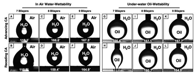
Fig. 5 (A-L) Advancing (A, C, E, G, I and K) and receding (B, D, F, H, J and L) contact angle images of both the beaded water (A-F, in air) and oil (G-L, under water) phases on the multilayers (7 bilayers: A and B, and G and H; 8 bilayers: C and D, and I and J; 9 bilayers: E and F, and K and L) of the NCs that were post chemically modified with ODA (A-F) and glucamine (G-L).
