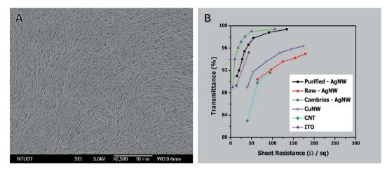
Fig. 8 (A) Typical FE-SEM image of AgNW film. (B) A plot of specular transmittance ( $\lambda = 550$  nm) *versus* sheet resistance for AgNW films before and after purification. Each data point is the average of five measurements. The performances of AgNWs,<sup>42</sup> CuNWs,<sup>94</sup> CNT,<sup>95</sup> and ITO are shown for comparison.
