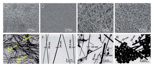
Fig. 3 FE-SEM (A-D) and TEM (E-H) images of purified products obtained from different concentrations of AgNO<sub>3</sub>: (A and E) 20.6, (B and F) 30.5, (C and G) 60.4 and (D and H) 90.3 mM respectively, while the other all parameters were kept constant.
