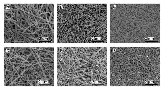
Fig. 4 FE-SEM images of AgNWs synthesized at different [PVP] to [AgNO<sub>3</sub>] molar ratio: (A) 2:1, (B) 4:1, (C) 6:1, (D) 8:1, (E) 10:1, and (F) 12:1.
