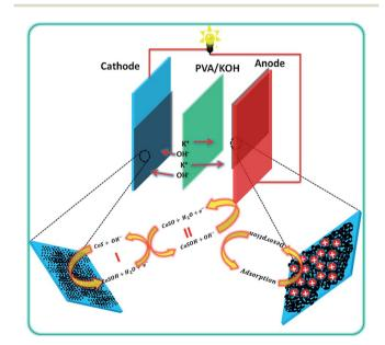
Fig. 6 Schematic of the flexible asymmetric supercapacitor fabrication with PVA/KOH-based all-solid-state electrolyte and their energy storage mechanism.
