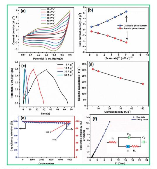
Fig. 4 (a) CV profile of the CoS electrode at different scan rates. (b) Peak current density as a function of scan rate. (c) CD profile of the CoS electrode at different current densities. (d) Specific capacitance of the CoS electrode as a function of current density. (e) Specific capacitance retention of the CoS electrode as a function of cycle number at 50 A g<sup>-1</sup>. (f) EIS analysis of the CoS electrode and corresponding equivalent circuit (inset) in a 20% KOH solution.
