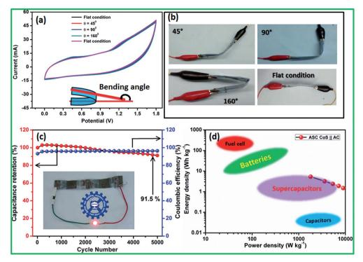
Fig. 8 (a) CV profile of the fabricated flexible ASC cell with different bending angles at a scan rate of 100 mV  $s^{-1}$ . (b) Image of the bent cells. (c) Specific capacitance and coulombic efficiency of the fabricated flexible ASC cell as a function of cycle number. (d) Typical Ragone plot of the fabricated flexible ASC cell and the location, where other energy storage devices would be located on the plot, is highlighted.
