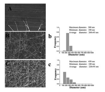
Fig. 3 SEM images of the electrospun nanofilm with different  $\beta$ -CD concentrations (A: 1%  $\beta$ -CD; B: 2%  $\beta$ -CD; and C: 3%  $\beta$ -CD) and fiber diameter distribution of the electrospun nanofilm (b: PVA/CEO/LYS/ 2% β-CD and c: PVA/CEO/LYS/3% β-CD).
