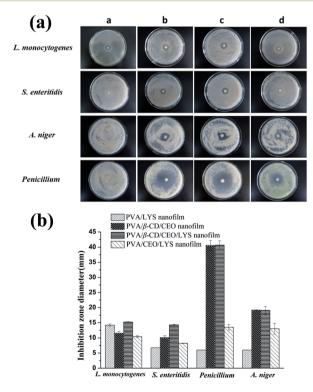
**Fig. 8** Inhibition zones (a) and the corresponding diameter (b) of different electrospun nanofilms against *L. monocytogenes, S. enteritidis, A. niger* and *Penicillium*. (a: PVA/LYS nanofilm; b: PVA/β-CD/CEO nanofilm; c: PVA/β-CD/CEO/LYS nanofilm; and d: PVA/CEO/LYS nanofilm).
