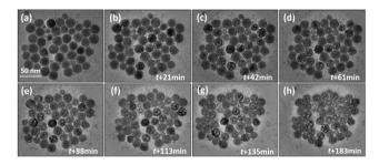
Fig. 2 (a-h) Time dependence of the morphology reconfiguration of NaGdF<sub>4</sub>:Yb,Er nanoparticles induced by 200 kV electron beam irradiation with the current density at 52 pA cm<sup>-2</sup>. The scale bar is
