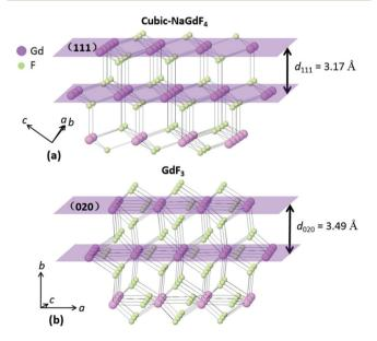
Fig. 7 Crystal structure for (a) cubic-NaGdF $_4$  adopting a face-centered symmetry with the stacking pattern of a (111) plane and for (b) GdF $_3$  adopting an orthorhombic symmetry with a stacking pattern of a (020) plane. Gd/Na atoms are indicated as purple spheres and F atoms as green ones.
