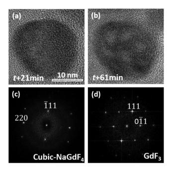
Fig. 3 TEM images of an individual NaGdF<sub>4</sub>:Yb,Er nanoparticle after electron beam irradiation for (a) 21 min and (b) 61 min with the current density at 52 pA cm<sup>-2</sup>, (c) and (d) show their corresponding FFT patterns labeled with Miller indices.
