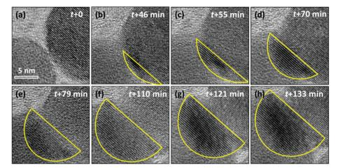
Fig. 4 (a-h) Time dependence of the in situ epitaxial growth of GdF<sub>3</sub> on NaGdF<sub>4</sub> at the interface induced by a focused electron beam with a current density of 40 pA cm $^{-2}$ . The scale bar in all figures is 5 nm. GdF<sub>3</sub> layers are marked with yellow lines for a guide to the eye.
