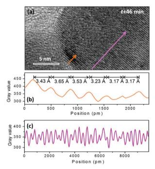
Fig. 5 (a) HRTEM image of the GdF<sub>3</sub>-NaGdF<sub>4</sub> interface at the irradiation time of 46 min. (b) and (c) Profiles of line scans along the GdF<sub>3</sub>-NaGdF<sub>4</sub> interface (orange arrow) and along the particle body of NaGdF<sub>4</sub> (111) (pink arrow).
