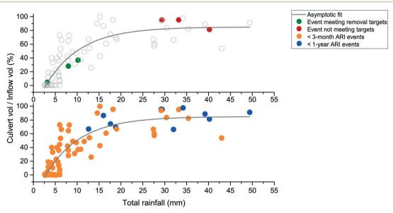
Fig. 3 Culvert discharge volume as percentage of total inflow volume, highlighting the water quality performance of the six sampled events (top) and categorization of events in the monitoring period into <3 month and <1 year ARI events (bottom) (adapted from Wang et al. 46).
