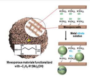
**Scheme 1** Selective precipitation of the metal nitrate precursors on the mesopore walls can be realized by functionalization of mesopore walls with  $-C_3H_6-N^+(Me)_3(OH)^-$  groups. Soluble metal precursors can be converted to insoluble metal hydroxyl species.
