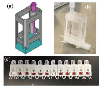
Fig. 3 A spotting apparatus was designed (a) and used to spot 12  $\mu L$  of blood onto the Prosolia paper spray cartridges (b, c).
