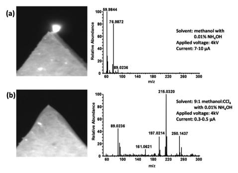
Fig. 4 (a) Photograph of the paper tip after application of high voltage and a typical mass spectrum when using methanol as a spray solvent. Corona discharge is indicated by the glowing spot in the photograph, the high spray current, and the ions detected that overwhelm the full-MS spectrum. (b) Photograph and mass spectrum obtained under identical conditions using 9:1 methanol: CCl4 as the spray solvent. The lower spray current as well as the visible Taylor cone indicate a stable electrospray.
