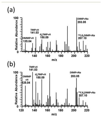
Fig. 1 PS-MS full scan mass spectra for 10 ppm TMP,  $d_9$ TMP, & DMMP; 2 ppm DIMP &  $^{13}$ Cd $_3$ DIMP spiked into blood (a) and urine (b). Data were collected in positive ion mode using 95/5 methanol/water with 0.01% formic acid.
