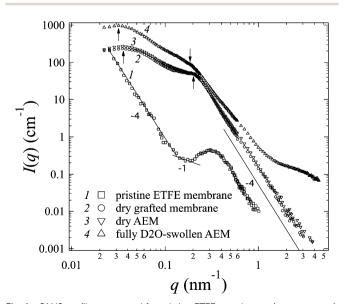
Fig. 1 SANS profiles measured for pristine ETFE membranes (open squares), grafted-ETFE (open circles), dry 2Me-AEMs (open down-triangles) and fully  $D_2O$  swollen 2Me-AEMs (open up-triangles) at room temperature.
