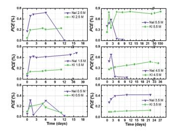
Fig. 5 PCE values as a function of time of aqueous DSSCs assembled with different  $I^-$  salts and at different concentrations, keeping  $I_2$  constant at 50 mM. Cells (stored at room temperature under dark conditions) were tested at 1 sun irradiation and the reported data were recorded at the  $3^{rd}$  J-V measurement. Lines simply connect data points for better reading and have no physical meaning.
