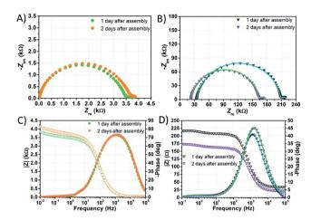
Fig. 7 EIS spectra of aqueous DSSCs assembled with KI 1.50 M + I $_2$  50 mM (A and C) and NaI 1.50 M + I $_2$  50 mM (B and D). Data points were fitted (lines) according to eqn (3) with the constraints  $R_{\rm Pt}=2~\Omega$  and  $C_{\rm Pt}=2~\chi~10^{-5}~{\rm F}$ .
