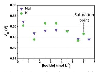
Fig. 3 Average  $V_{oc}$  values recorded one day after cell assembly.  $I_2$  was kept constant at 50 mM for all the cells. Data are referred to the 3<sup>rd</sup> measurement under 1 sun irradiation. Data referred to the electrolytes saturated with KI were arbitrarily placed at 6 M.
