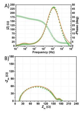
Fig. 9 Phase (filled circles) and modulus (open circles) Bode (A) and Nyquist (B) plots of the dummy cell filled with aqueous electrolyte comprised of KI 1.50 M + I $_2$  50 mM. Data points, recorded five months after cell assembly, were fitted (lines) according to eqn (3) with the constraint  $R_{Pt}=2~\Omega$  and  $C_{Pt}=2~\times~10^{-5}~\text{F}.$
