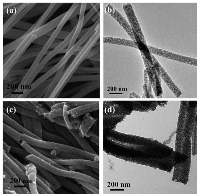
Fig. 5 (a) FESEM and (b) TEM micrograph of TiO<sub>2</sub> nanofibers; (c) FESEM and (d) TEM micrograph of TiO<sub>2</sub>–wsCQDs composites.
