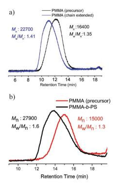
Fig. 4 Comparison of the GPC traces of precursor PMMA with (a) chain extended PMMA and (b) PMMA-b-PS before.
