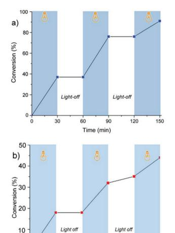
Fig. 2 Monomer conversion (%) vs. time using erythrosin B (a) and eosin Y (b) to determine the dependency of propagation on irradiation: light on (blue regions) light off (white regions).
