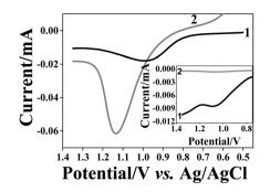
**Fig. 6** LSV recorded in 0.1 M KCl for NAIMs formed by ITO/PEI/10 nm AuNP/PAA after reuptake of 10 nm (curves 1) and 40 nm (curves 2) AuNPs for 1 h. The inset compares the curves after the currents were normalized to the particle volumes: for 10 nm AuNPs (curve 1) the current was divided by 1 and for 40 nm AuNPs (curve 2) the current was divided by 64.
