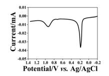
**Fig. 8** Oxidation of AgNPs and AuNPs reuptaken (1 h) from a NP mixture by the ITO/PEI/PAA NAIMs after oxidative removal of the 10 nm template AuNPs. LSV was recorded in 0.1 M KCl.
