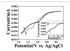
**Fig. 7** LSV recorded in 0.1 M KCl for ITO/PEI/10 nm AuNPs/PAA/1-hexadecylamine NAIM after reuptake of 10 nm (curves 1) and 40 nm (curves 2) AuNPs for 1 h. The inset compares the curves after the currents were normalized to the particle volumes. The currents were divided by 1 (curve 1) and 64 (curve 2) for the 10 and 40 nm AuNPs, respectively.
