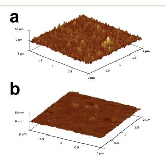
**Fig. 3** AFM images of topography changes of ITO/PEI/AuNPs/PAA before (a) and after (b) electrooxidation of AuNPs. LSV between 0.6 V and 1.3 V at 0.05 V s<sup>-1</sup>. X- and Y-axes max = 2  $\mu$ m, Z-axes max = 50 nm.
