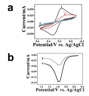
**Fig. 4** Electrochemical characterization of ITO/PEI/AuNPs/PAA: (a) CV of the ITO electrode covered with a PAA matrix: (1) before and (2) after AuNP oxidation; (3) after AuNPs reuptake and (4) after the second oxidation. Experiments were carried out in 1 mM  $[Fe(CN)_6]^{4-}$  at 0.1 M KCl. (b) LSV of (1) template AuNP oxidation and (2) oxidation of reuptaken AuNPs in 0.1 M KCl at a scan rate of 0.05 V s<sup>-1</sup>.
