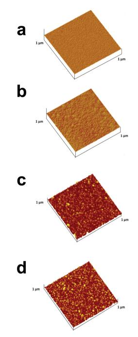
Fig. 1 AFM images of sequentially assembled NAIM systems on Si wafers: (a) bare Si, (b) Si after treatment with PEI (1 h), (c) followed by AuNP adsorption for 2 h, and (d) after adsorbing OA for 1 h. Z-Axes max = 25 nm.
