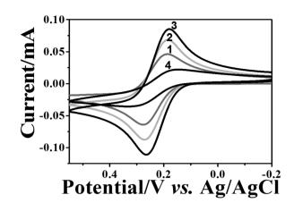
**Fig. 2** Electrochemical characterization of the step-by-step film assembly. CV recorded in 1 mM [Fe(CN)<sub>6</sub>]<sup>4–</sup> and 0.1 M KCl at (1) bare ITO; (2) after treatment with PEI; (3) after adsorption of AuNPs; and (4) after treatment with OA. The scan rate was 0.05 V s<sup>-1</sup>.
