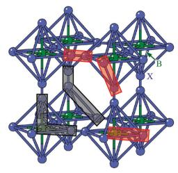
Representation of the simplified molecular perovskite structure used in our lattice-dynamical model. B atoms (shown in green) are located at the origin of the Pm3m cell, and X atoms (shown in blue) are located on the 6e site. The network is held together by a combination of harmonic bond stretching potentials (relevant pairs highlighted in red) and bond angle potentials (relevant triplets highlighted in black).
