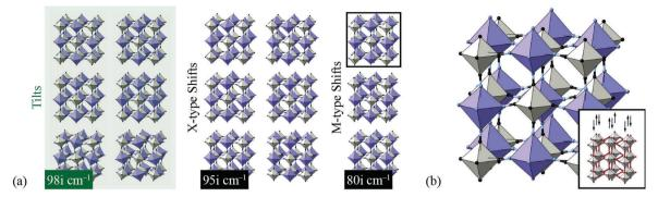
Fig. 11 Key zone-centre displacive instabilities in  $CdPd(CN)_6$  as determined using DFT calculations. (a) Conventional tilts (highlighted in green) are the least stable modes, followed by X-type and M-type shifts. (b) A representation of the phonon eigenvector associated with one of the M-type shift instabilities (highlighted in panel (a)), together with a schematic relating the collective displacements to the cartoon shown in Fig. 2(a).
