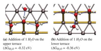
Fig. 2 Fully covered step edge with one additional water molecule on the Pt(533) step edge.
