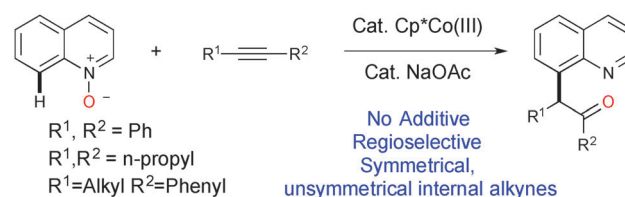
Scheme 1 Co(III) catalyzed C–H activation/oxygen atom transfer process.
