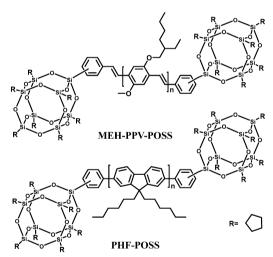
Chemical structures of MEH-PPV-POSS and PHF-POSS
