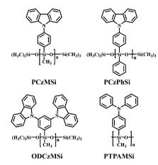
Fig. 22 Chemical structures of hole-transporting linear polysiloxane hosts.
