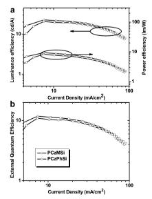
Fig. 23 (a) Luminance efficiency and power efficiency versus current density of PCzMSi and PCzPhSi. (b) External quantum efficiency versus current density of PCzMSi and PCzPhSi.
