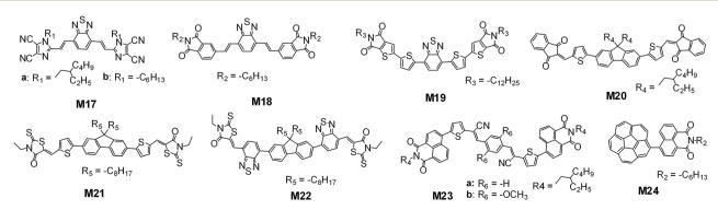
Fig. 13 Chemical structures of the reported typical small  $\pi$ -aromatic conjugation based small-molecule acceptors.
