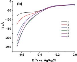
Fig. 6 Square wave voltammograms of (U, Pu)C FBTR sample on rGO/GC for (a) anodic scan from 0.35 V to 0.75 V for analyzing Pu and (b) cathodic scan from 0 V to -0.65 V for analyzing U. Square wave amplitude =25 mV; square wave frequency =20 Hz; step potential increment =1 mV; standby time at 0.35 V (for a) and at 0 V (for b) is 10 s. The numeric represents the sequence of the replicate measurements.
