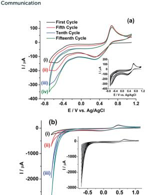
Fig. 7 Cyclic voltammograms of (U, Pu)C FBTR fuel sample on (a) rGO/GC and (b) GC electrodes at a scan rate of 50 mV s $^{-1}$  for (i) first, (ii) fifth, (iii) tenth and (iv) fifteenth cycle. The insets show the continuous cyclic voltammograms of 15 cycles.
