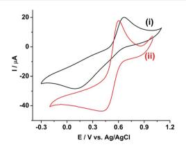
Fig. 1 Cyclic voltammograms of 10 mM Pu( $_{\rm IV}$ ) in 1 M H<sub>2</sub>SO<sub>4</sub> solution on (i) GC and (ii) rGO/GC electrodes at a scan rate of 10 mV s<sup>-1</sup>.
