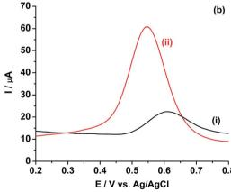
Fig. 4 Square wave voltammograms of 10 mM Pu(IV) in 1 M  $H_2SO_4$  solution on (i) GC and (ii) rGO/GC electrodes in the (a) cathodic and (b) anodic scan directions. Square wave amplitude = 25 mV; square wave frequency = 20 Hz; step potential increment = 1 mV; hold time at initial potential = 10 s.
