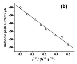
Fig. 2 (a) Cyclic voltammograms of 10 mM Pu(v) in 1 M H $_2$ SO $_4$  solution on GC electrode at a scan rate (v) of (i) 10, (ii) 25, (iii) 50, (iv) 75, (v) 100, (v) 150, (v) 200 and (v) 250 mV s $^{-1}$ . The inset shows the plots of  $\ln(I_p)$  versus  $\ln(v)$  for (1) cathodic and (2) anodic peaks. (b) Plot of the cathodic peak current versus the square root of the scan rate ( $v^{1/2}$ ).
