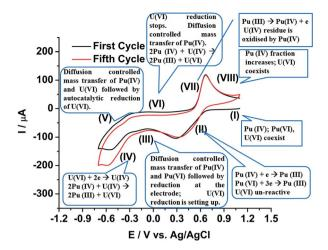
Fig. 9 Comprehensive representation of the autocatalytic reduction of U(vi) in the FBTR fuel sample solution containing both uranium and plutonium in 1 M H<sub>2</sub>SO<sub>4</sub>.
