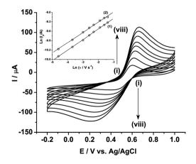
Fig. 3 Cyclic voltammograms of 10 mM Pu( $_{\rm IV}$ ) in 1 M H $_{\rm 2}$ SO $_{\rm 4}$  solution on rGO/GC electrode at a scan rate ( $_{\rm V}$ ) of (i) 10, (ii) 25, (iii) 50, (iv) 75, (v) 100, (vi) 150, (vii) 200 and (viii) 250 mV s $^{-1}$ . The inset shows the plots of  $\ln(I_p)$  versus  $\ln(v)$  for (1) cathodic and (2) anodic peaks.
