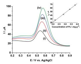
Fig. 5 ASWVs of (i) 2.17, (ii) 2.86, (iii) 3.38 and (iv) 3.81 mg g<sup>-1</sup> of Pu in 1 M H<sub>2</sub>SO<sub>4</sub> on rGO/GC. Square wave amplitude = 25 mV; square wave frequency = 20 Hz; step potential increment = 1 mV; hold time at initial potential = 10 s. Inset shows the sensitivity plot for the same. The vertical bars shown in the inset represent the standard deviation ( $\sigma$ ) of  $I_p$  obtained from ten replicate measurements for each concentration of Pu.
