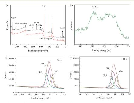
Fig. 7 Wide XPS spectra of (a) CoFe<sub>2</sub>O<sub>4</sub>/MgAl-LDH before and after Cr(vi) adsorption, (b) Cr 2p spectrum of CoFe<sub>2</sub>O<sub>4</sub>/MgAl-LDH after Cr(vi) adsorption, (c) O 1s spectrum of CoFe<sub>2</sub>O<sub>4</sub>/MgAl-LDH, and (d) O 1s spectrum of CoFe<sub>2</sub>O<sub>4</sub>/MgAl-LDH after Cr(vi) adsorption.
