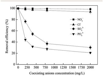
Fig. 9 Effect of coexisting anions on adsorption of Cr(vı) on CoFe $_2$ O $_4$ / MgAl-LDH.
