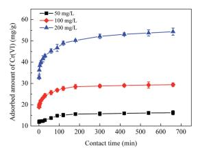
Fig. 3 Effect of contact time on  $Cr(v_1)$  adsorption using  $CoFe_2O_4/MqAl-LDH$  for initial  $Cr(v_1)$  concentrations of 50, 100 and 200 mg  $L^{-1}$ .
