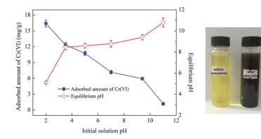
$\label{eq:Fig. 2} \textbf{ Effect of initial solution pH on } Cr(vi) \textbf{ adsorption and equilibrium pH using } CoFe_2O_4/MgAl-LDH.$
