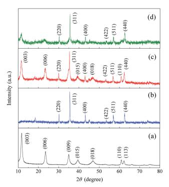
Fig. 1 XRD patterns of (a) MgAl-LDH, (b) CoFe $_2$ O $_4$ , (c) CoFe $_2$ O $_4$ /MgAl-LDH, and (d) CoFe $_2$ O $_4$ /MgAl-LDH after Cr( $_1$ ) adsorption.
