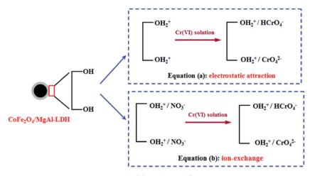
Fig. 8 Schematic illustration of the adsorption mechanism of Cr(vi) on CoFe<sub>2</sub>O<sub>4</sub>/MgAl-LDH.
