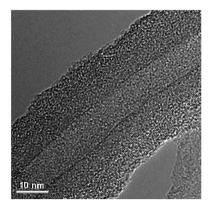
Fig. 9 High resolution TEM images of the MWCNT@PPy-MnO<sub>2</sub> coreshell structure. Reproduced with permission from ref. 92. Copyright 2009 Elsevier.
