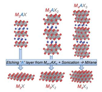
Fig. 14 Schematic of the fabrication of MXene. Reproduced with permission from ref. 162. Copyright 2013 WILEY-VCH Verlag GmbH & Co. KGaA, Weinheim.
