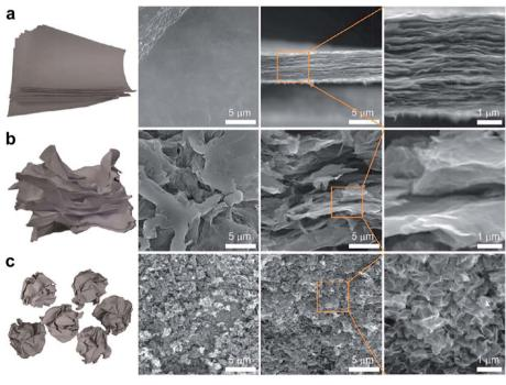
Fig. 18 Paper models and SEM images showing stacks of (a) flat graphene sheets, (b) heavily wrinkled sheets, and (c) crumpled graphene balls. Reproduced with permission from ref. 222. Copyright 2013 American Chemical Society.
