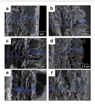
Fig. 21 Cross-section morphologies and X-ray line scan spectra of Mn element in pristine composites (MCM0), and after 500 cycles at 20 mV s $^{-1}$ (MCM20), 60 mV  $s^{-1}$  (MCM60), 100 mV  $s^{-1}$  (MCM100), 300 mV  $s^{-1}$ (MCM300), and 500 mV  $s^{-1}$  (MCM500). (a) MCM0, (b) MCM20, (c) MCM 60, (d) MCM100, (e) MCM300, and (f) MCM500. Reproduced with permission from ref. 232. Copyright 2012 Elsevier.
