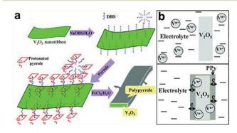
Fig. 10 (a) Schematic shows the growth of PPy on V<sub>2</sub>O<sub>5</sub> nanoribbon surface. (b) PPy shell helps the electronic transport and prevents the dissolution of vanadium in electrolyte. Reproduced with permission from ref. 103. Copyright 2013 WILEY-VCH Verlag GmbH & Co. KGaA, Weinheim.
