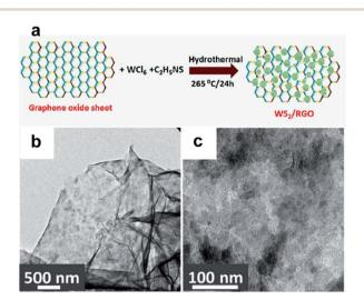
Fig. 16 (a) Hydrothermal synthesis of the  $WS_2$ -rGO materials. (b and c) TEM images of the resulting  $WS_2$ -rGO electrode material. Reproduced with permission from ref. 183. Copyright 2013 American Chemical Society.
