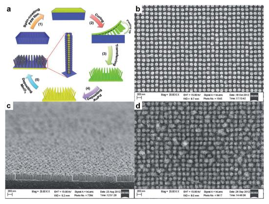
Fig. 7 (a) Schematic illustration of the development of MnO2 coated electrodes. SEM images show top (a) and side (b) view of as-printed PAN nanostructures. (d) SEM image of electrochemically deposited MnO<sub>2</sub> nanoparticulates on pillar nanoarrays. Reproduced with permission from ref. 52. Copyright 2013 WILEY-VCH Verlag GmbH & Co. KGaA, Weinheim.
