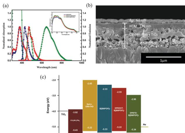
Fig. 2 (a) Absorption and emission spectra of the HTMs in chlorobenzene. Inset: UV-vis absorption spectra of the HTMs coated on mp-TiO<sub>2</sub>/MAPbI<sub>3</sub> films. (b) Cross-sectional field-emission scanning electron microscopy (FE-SEM) image of mp-TiO<sub>2</sub>/MAPbI<sub>3</sub>/HTM/Au. (c) Energy level diagram of each component.
