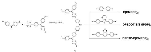
Scheme 1 Schematic diagram for the synthesis of **B[BMPDP]<sub>2</sub>**, **DPEDOT-B[BMPDP]<sub>2</sub>** and **DPBTD-B[BMPDP]<sub>2</sub>**.
