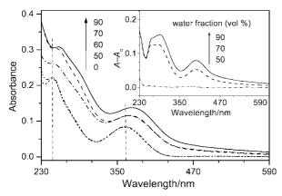
Fig. 3 UV spectra of 1 in water–ethanol mixtures (concentration of 1: 10  $\mu$ M). Inset: differential spectra of 1 (*A* and  $A_0$  being absorbance of 1 in mixture solvent and absolute ethanol, respectively).
