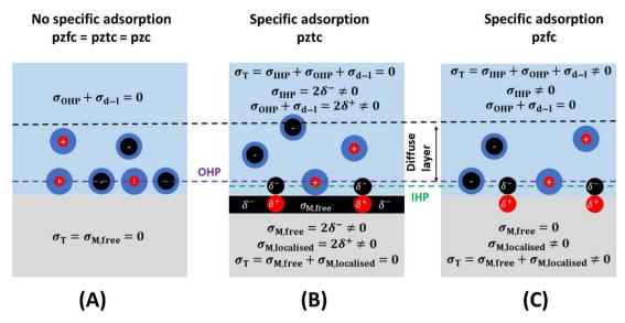
Fig. 3 The pzfc and the pztc. In the absence of specific adsorption (A), the pztc and the pzfc coincide. When there are specifically adsorbed species on the metal surface (B and C), the free charge density on the metal surface is not zero at the pzfc (B), while the total charge density is not zero at the pzfc (C).
