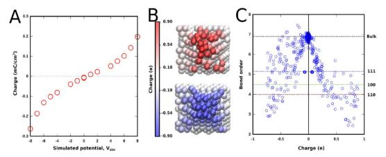
Fig. 7 (A) Charge accumulation upon application of an external simulated voltage ( $V_{\text{sim}}$ ). (B) Snapshot showing charge accumulation on the polycrystalline protruding electrode at  $\pm 7V_{\text{sim}}$ . (C) Bond order dependence of charge accumulated on the surface atoms on both electrodes at a bias of  $\pm 7V_{\text{sim}}$ .
