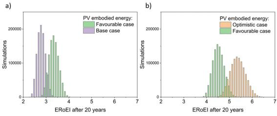
Fig. 4 Histograms of ERoEI after 20 years setting the PV embodied energy at the indicated bounds and selecting all other parameters at random within their specified ranges (defined in Table 1) for (a) between the base and favourable cases, and (b) between the favourable and optimistic cases; 1000 000 simulations for each profile.
