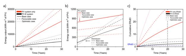
Fig. 2 Energy metrics over time for simulated PV facilities (red traces) and PV-coupled electrolyser facilities (black traces) for (a) output energy production, (b) energy input costs, and (c) ERoEI for electricity and hydrogen production. The shaded envelopes show the range in the favourable to unfavourable parameters about the base-case simulation
