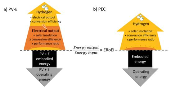
Fig. 1 Schematic of the parameters for calculating the ERoEl over time for (a) a PV-E facility and (b) a PEC facility. ERoEl is the ratio of calculations above and below the line
