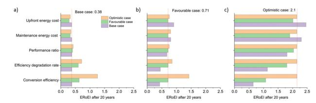
Fig. 6 Sensitivity analysis for parameters affecting the PEC facility starting at (a) the base-case scenario (ERoEI of 0.38), (b) the favourable-case scenario (ERoEI of 0.71), and (c) the optimistic-case scenario (ERoEI of 2.1).
