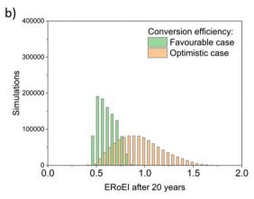
Fig. 7 Histograms of the EROEI after 20 years for a modelled PEC facility with conversion efficiency (CE) indicated; 1000 000 simulations each profile, (a) randomised parameters between the base case and favourable case, (b) randomised parameters between the favourable case and optimistic case.
