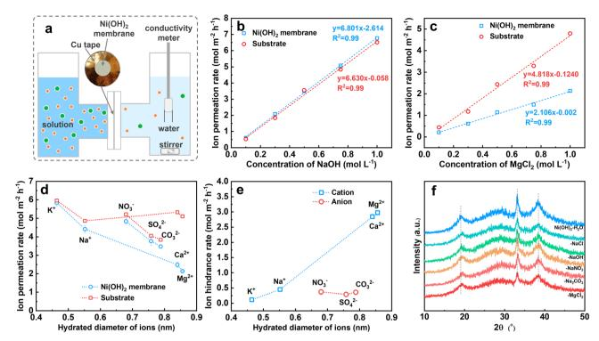
Fig. 4 (a) Schematic of Ni(OH)<sub>2</sub> membrane test setup. Ion permeation rates under different concentrations of (b) NaOH and (c) MgCl<sub>2</sub> solutions. (d) Ion permeation rate versus ion hydrated diameter of the substrate and Ni(OH)2-membrane-coated substrate. (e) The calculated ion hindrance rate for the Ni(OH)<sub>2</sub> membrane. (f) XRD patterns of Ni(OH)<sub>2</sub> membrane powder after immersion in different solutions.
