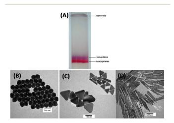
**Fig. 4** (A) Digital image of preparative agarose gel electrophoretic column shows the separated nanospheres (red band), nanoplates (blue band) and long nanorods (light brown band), TEM images of (B) separated pure nanospheres, (C) separated nanoplates (inset shows some short rods coexist with plates), and (D) purified long gold nanorods. This figure has been reproduced from ref. 50 with permission from Elsevier, copyright 2005.
