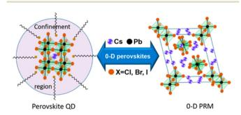
Fig. 9 Schematic representation of two types of 0-D perovskites. Perovskite QDs with general formulas of ABX<sub>3</sub> and size less than the exciton Bohr diameter (represented by the circle) and 0-D perovskiterelated materials with spatially isolated octahedra in a bulk crystal lattice. This figure has been reproduced from ref. 88 with permission from the American Chemical Society, copyright 2018.
