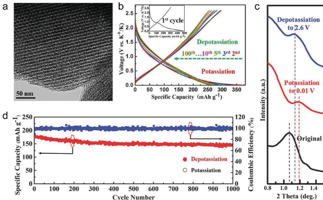
Fig. 23 (a) TEM, (b) the 2nd, 3rd, 5th, 10th, 20th, 30th, 50th, 75th, and 100th potassiation/depotassiation profiles, (c) *ex situ* XRD patterns, and (d) long-term cycling stability and CE of the mesoporous carbon. Reproduced from ref. 80 with permission from Wiley-VCH.
