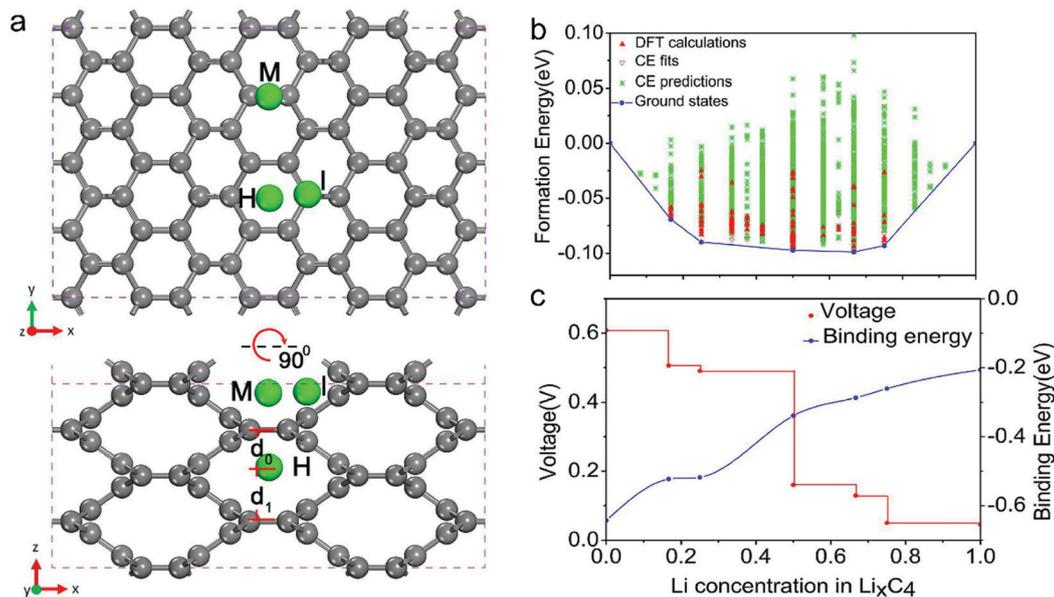
Fig. 16 (a) Structure of bco-C<sub>16</sub> and the schematics of the possible Li-ion absorption sites in top and side view. (b) Formation energies predicted for the 150 different Li configurations with 5 stable intermediate phases. (c) Corresponding voltage profile (marked in red) and binding energy profile (marked in blue) calculated along the minimum energy path. Reproduced from ref. 298 with permission from United States National Academy of Sciences.
