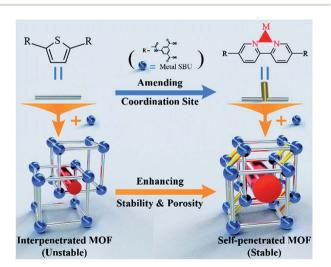
Fig. 7 Schematic diagram showing the framework and the modification strategy. The blue-colored balls, silver-colored sticks, yellowcolored sticks, and red-colored cylinders represent metal SBUs, ligands, coordinate bonds and pores, respectively. Reproduced from ref. 124 with permission from The Royal Society of Chemistry, copyright 2018.
