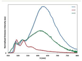
Fig. 9 Solid-state emission spectra of complexes 1-3. The emission profiles have been normalised on the principal <sup>3</sup>LC band for each complex.
