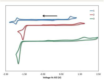
Fig. 4 CV traces of 1-3 in MeCN solution, reported *versus* SCE (Fc/Fc<sup>+</sup> = 0.38 V in MeCN).<sup>29</sup> Scans are in the negative scan direction at a scan rate of 100 mV s<sup>-1</sup>.
