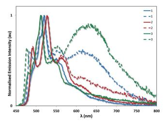
Fig. 10 Powder emission spectra of complexes 1–3 before (solid lines) and after grinding (dashed lines). The emission profiles have been normalised on the principal <sup>3</sup>LC band for each complex.
