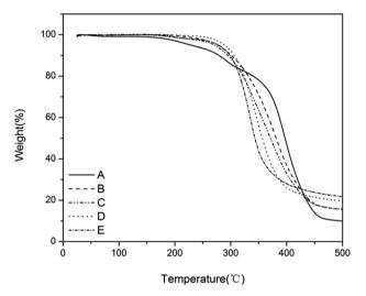
TGA curve of the films with a charge density gradient. (A) T:D=1:0, (B) T:D=2:1, (C) T:D=1:1, (D) T:D=1:2 and (E) T:D=1:1
