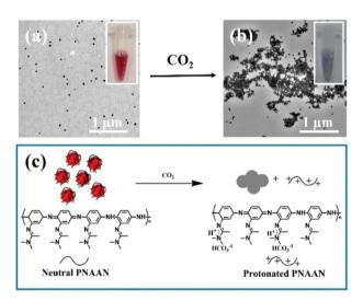
Fig. 3 TEM images of AuNPs (a) before and (b) after being purged with  $CO_2$  gas. (c) Schematic illustration of  $CO_2$  induced AuNP aggregation. Insets of (a) and (b) show photographs of the AuNP solutions (a) before and (b) after being purged with  $CO_2$  gas. Reprinted with permission from ref. 69. Copyright 2016, American Chemical Society.
