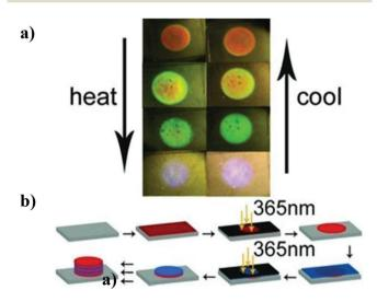
Fig. 6 (a) Photographs of a sensor changing color as a function of temperature-heating induces deswelling, while cooling induces swelling. (b) Schematic representation of sensor fabrication (red layers, PpMS; blue layers, pNIPAm-co-AAc). Reprinted with permission from ref. 79. Copyright 2012, Wiley-VCH Verlag GmbH & Co. KGaA.
