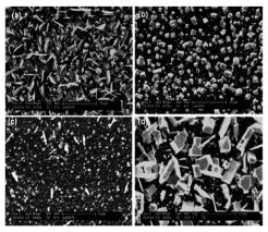
Fig. 11 SEM of PbS thin films deposited from [Pb(S<sub>2</sub>CNMeBenzyl)<sub>2</sub>]. At (a) 375 °C, (b) 425 °C, (c) 475 °C and (d) 525 °C. Reproduced from ref. 102 with permission from The Royal Society of Chemistry.
