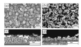
Fig. 14 SEM of  $Bi_2S_3$  thin films deposited *via* AACVD from  $[Bi(S_2CNEt_2)_3]_2$  in chloroform/toluene at (a) 400 °C, (b) 450 °C, (c) and (d) show cross-section of films deposited at 400 and 450 °C, respectively. Reproduced with permission from ref. 114. Copyright 2014 American Chemical Society.
