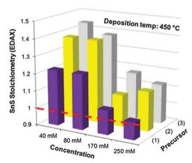
**Fig. 9** The effect of concentration of precursors where (1) is  $[Sn(S_2CNEt^nBu)_2]$ , (2) is  $[Sn(S_2CNEt^nBu)_2]$  and (3) is  $[Sn(S_2CNEt_2)_2]$  on the stoichiometry (%Sn divided by %S found experimentally by EDAX) of SnS films deposited at 450 °C by AACVD. The dashed line indicates an ideal 1:1 Sn:S stoichiometry *i.e.* SnS. Reproduced with permission from ref. 98. Copyright 2014 Elsevier.
