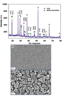
Fig. 35 XRD pattern of monoclinic BiVO<sub>4</sub> (green) on FTO (red) coated glass substrate deposited *via* AACVD; below: SEM image of BiVO<sub>4</sub> thin film at (a)  $20\,000\times$  and (b)  $100\,000\times$ . Reproduced with permission from ref. 248. Copyright 2012 Wiley.
