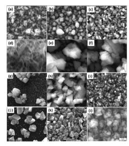
**Fig. 8** SEM images of β-ln<sub>2</sub>S<sub>3</sub> films deposited using the precursors  $[ln(S_2CNCy_2)_3]\cdot 2py$  at (a) 300 °C, (b) 350 °C and (c) 400 °C;  $[ln(S_2CN(Pr)_2)_3]\cdot 1.5py$  at (d) 300 °C, (e) 350 °C and (f) 400 °C;  $[ln(S_2CNPp)_3]\cdot 0.5py$  at (g) 300 °C (h), 350 °C and (i) 400 °C and  $[ln(S_2CNBzMe)_3]$  at (j) 300 °C, (k) 350 °C and (l) 400 °C. Reproduced from ref. 85 with permission from The Royal Society of Chemistry.
