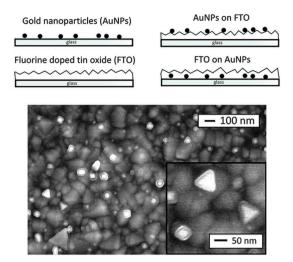
Fig. 28 Top: Schematic of layers deposited. Bottom: SEM image of AuNPs (from  $0.5 imes 10^{-2}$  mmol auric acid) deposited onto a bottom plate of FTO. Reproduced from ref. 215 with permission from The Royal Society of Chemistry.
