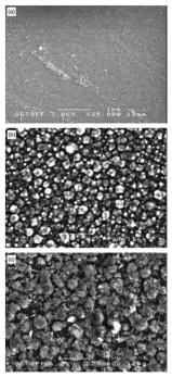
Fig. 24 SEM of films grown from AACVD deposition of InMe<sub>3</sub> and MeOH at (a) 400 °C; (b) 450 °C; and (c) 500 °C. Reproduced with permission from ref. 176 Copyright 2013 Royal Australian Chemical Institute
