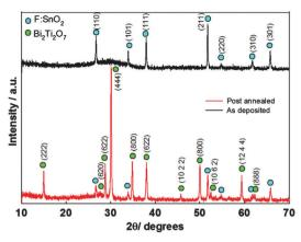
Fig. 34 X-ray diffraction pattern of the as-deposited (black) and post-annealed (red)  ${\rm Bi_2Ti_2O_7}$  thin film. Reproduced with permission from ref. 247. Copyright 2014 Elsevier.
