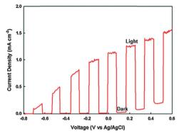
Fig. 36 J-V plot of In<sub>2</sub>S<sub>3</sub> films obtained from AACVD at 400 °C from [In(S<sub>2</sub>CN<sup>i</sup>Pr<sub>2</sub>)<sub>3</sub>·1.5(py)]. Reproduced with permission from ref. 85. Copyright 2013 Royal Society of Chemistry
