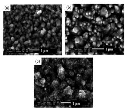
**Fig. 4** SEM images of CdS thin films deposited from  $[Cd(S_2CNC_5H_{10})_2\cdot py]$  at (a) 350 °C; (b) 400 °C and (c) 450 °C. Reproduced from ref. 40 with permission from the Centre National de la Recherche Scientifique (CNRS) and the Royal Society of Chemistry.
