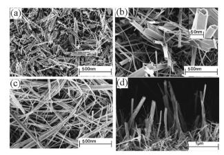
Fig. 13 SEM of  $Bi_2S_3$  deposited *via* AACVD from  $[Bi(S_2CNEt_2)_3]_2$  in chloroform at (a) 350 °C, (b) 400 °C, (c) 450 °C and (d) cross-section of film deposited at 400 °C. The inset of (b) shows a high resolution image of a nanotube. Reproduced with permission from ref. 114. Copyright 2014 American Chemical Society.
