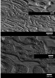
Fig. 5 SEM images of crystalline GaAs films grown via AACVD from As(NMe<sub>2</sub>)<sub>3</sub> and GaMe<sub>3</sub> at (a) 500 °C and (b) 550 °C. Reproduced from ref. 63 with permission from The Royal Society of Chemistry.
