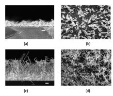
Fig. 32 SEM of the films grown from [Bi(O<sub>2</sub>CN<sup>i</sup>Pr<sub>2</sub>)<sub>3</sub>], (a and b) at 300 °C for 40 minutes, and (c and d) at 450 °C for 40 minutes. Reproduced with permission from ref. 244. Copyright 2013 American Chemical Society.
