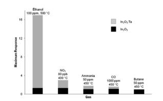
Fig. 37 Maximum gas response of In<sub>2</sub>O<sub>3</sub> and In<sub>2</sub>O<sub>3</sub>:Ta sensors to different gases in flowing air at optimum operating temperatures. Reproduced with permission from ref. 256. Copyright 2012 American Chemical Society.
