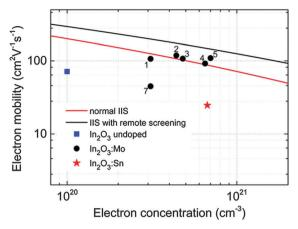
Fig. 26 Electron mobility and concentration for undoped, Sn-doped and Mo-doped  $\ln_2 O_3$ . The numbers by the data points correspond to the mol% of Mo dopant in the solution used in the AACVD. The model curves for regular ionized impurity scattering (IIS) (red line) and for remotely screened IIS (black line). All calculations are for singly ionized Mo donor atoms. Reproduced with permission from ref. 193. Copyright 2015 American Chemical Society.
