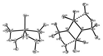
Fig. 18 Crystal structure of: left, [Ga(OCH(CH<sub>3</sub>)CH<sub>2</sub>NMe<sub>2</sub>)<sub>2</sub>Cl], right, [Ga(OC(CH<sub>3</sub>)<sub>2</sub>CH<sub>2</sub>OMe)Cl<sub>2</sub>]<sub>2</sub> both with thermal ellipsoids shown at the 50% probability level (hydrogen atoms omitted for clarity). Reproduced from ref. 153 with permission from the Centre National de la Recherche Scientifique (CNRS) and the Royal Society of Chemistry.
