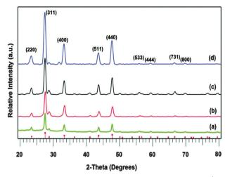
Fig. 6 p-XRD patterns of as deposited In<sub>2</sub>S<sub>3</sub> thin films from In[(S<sub>2</sub>P<sup>i</sup>Bu<sub>2</sub>)<sub>3</sub>] precursor at temperatures (a) 350 °C, (b) 400 °C, (c) 450 °C and (d) 500 °C. Vertical lines below show the standard ICDD pattern 01-084-1385 for In<sub>2</sub>S<sub>x</sub>, Reproduced from ref. 82 with permission from the Centre National de la Recherche Scientifique (CNRS) and the Royal Society of Chemistry.
