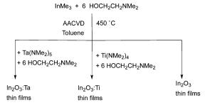
Scheme 5 Deposition of In<sub>2</sub>O<sub>3</sub> and In<sub>2</sub>O<sub>3</sub>:M via AACVD
