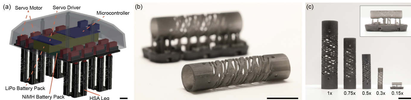
Fig. 1 3D Printed HSAs for Untethered Soft Robots. (a) A CAD rendering of the untethered soft robot shows the overall assembly, including four HSA-based legs, 16 servo motors, and on-board electronics and batteries enclosed within the robot's shell. (b) Photographs of a miniature HSA (0.3x scaling) show the part before (out-of-focus, in the background) and after processing (foreground). (c) 3D printed HSAs are shown at 1x, 0.75x, 0.5x, 0.3x, and 0.15x scalings. The inset in the upper right corner is a magnified view of the 0.15x HSAs, which can be printed but with supports that are difficult to remove without damaging the HSA. Scale bars are 20mm (a,c) and 10mm (b).
