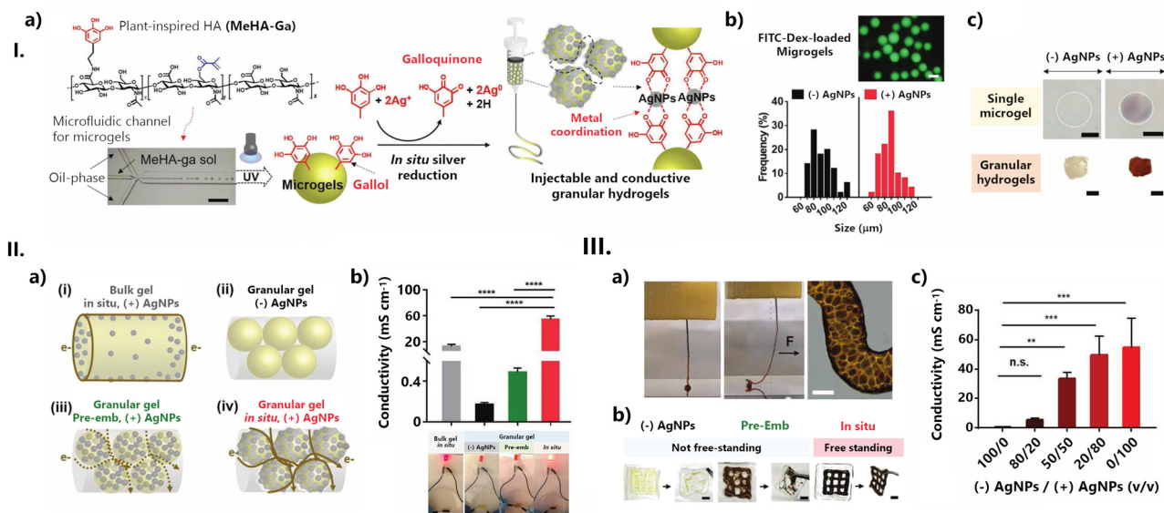
Fig. 30 (I) Fabrication of conductive granular hydrogels and their characterization. (a) Schematic of the preparation of conductive granular hydrogels using a microfluidic device to form microgels (formed with methacrylated and gallol-modified HA, MeHA-Ga) through a water-in-oil emulsion, in situ metal reduction by GA moieties, and then jamming through vacuum filtration. (b) Size distribution of microgels without ((-)AgNPs, black) or with ((+)AgNPs, red) AgNPs. The fluorescent image shows the microgels with encapsulated FITC-dextran for visualisation. Scale bar: 100 \mu\text{m} . (c) Optical images of single microgels (top) or granular hydrogels (bottom) either without ((-)AgNPs) or with ((+)AgNPs) in situ metal reduction. The colour change is due to the introduction of silver nanoparticles. A scale bar of 50 \mu\text{m} for top images and 3 mm for bottom ones. (II) Conductivity of granular hydrogels. (a) Schematic of hydrogel structures, including: (i) bulk hydrogels with AgNPs through the in situ process (" in situ "), (ii) granular hydrogels without AgNPs, (iii) granular hydrogels with AgNPs pre-embedded during microgel fabrication (" pre-emb "), or (iv) granular hydrogels with AgNPs through the in situ process. The brown line describes the proposed electron ( e^- ) transfer passing through each hydrogel, including a solid line for continuous flow and a dashed line for discontinuous flow. (b) Electrical conductivity in various hydrogels. One-way ANOVA, Dunnett's test for multiple comparisons to " in situ " microgels, ****p < 0.0001 . (c) LED-emitting tests in an electrical circuit serially connected with various hydrogels, showing the greatest light intensity for granular hydrogels with microgels treated with the " in situ " process. (III) 3D printing of conductive hydrogels. (a) Images of the 3D printing process of the conductive granular hydrogels and the morphology of the printed filament. The black arrow indicates a physical force (F) applied to the filament with needle translation during printing, showing the filament's self-support. (b) Printability of the granular hydrogels fabricated from microgels without AgNPs ("(-)AgNPs") or with pre-embedded (" pre-Emb ") or in situ synthesised (" in situ ") AgNPs on the polymeric film and their free-standing stability when removed with forceps. (c) Conductivity of extruded filaments as a function of volumetric mixing ratio v/v of the "(-)AgNPs" or " in situ , (+)AgNPs" microgels. One-way ANOVA, Dunnett's test for multiple comparisons to "100/0" filament, n.s. for not significant, **p < 0.01 , ***p < 0.001 . Scale bars: 100 \mu\text{m} for (a) and 3 mm for (b). Reproduced with adaptations from ref. 292; copyright © 2019 The Author(s). Published by Wiley-VCH Verlag GmbH & Co. KGaA, Weinheim. This work is licensed under a Creative Commons Attribution 4.0 CC-BY International License.
