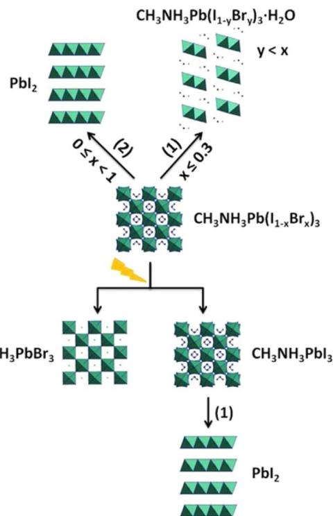
Fig. 5 Diagram of degradation of MAPb(I<sub>1-x</sub>Br<sub>x</sub>)<sub>3</sub> exposed to humidity.<sup>151</sup>
