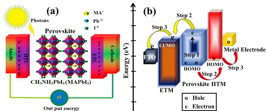
Fig. 2 (a) Working of PSCs and generation of electron–hole pairs in semiconductors, (b) energy levels in PSCs.<sup>36</sup>
