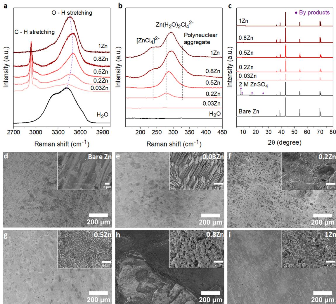
**Fig. 1** Electrolyte structure and Zn foil stability: (a) and (b) Raman spectra of WISEs corresponding to the water region and Zn coordination, respectively. (c) XRD patterns of the Zn foil before and after immersing in different WISEs for 10 days at room temperature, compared with diluted 2 M ZnSO<sub>4</sub>. SEM images of (d) bare Zn foil and Zn foil soaked in (e) 0.03Zn, (f) 0.2Zn, (g) 0.5Zn, (h) 0.8Zn, and (i) 1Zn WISEs.
