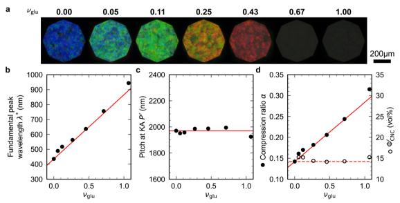
Fig. 6 (a) POM images (LCP reflection) for photonic CNC films with increasing glucose: CNC volume ratio,  $\nu_{\text{glu}}$ . (b) –(d) Fitting parameters ( $\lambda^*$ , P',  $\alpha$ ) for the CNC-glucose films. In (d) solid circles correspond to  $\alpha$ , and open circles correspond to  $\Phi'_{\text{CNC}}$  calculated using eqn (16). Red lines in (b)–(d) show the predicted trends for the reduced compression model (eqn (17) and (18)) with P'=1970 nm and  $\alpha_0=\Phi'_{\rm CNC}=0.142$ .
