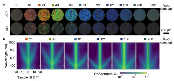
Fig. 3 (a) Polarised optical microscopy (POM) in reflection mode for photonic CNC films with increasing NaCl: CNC ratio  $\hat{c}_{NaCl}$ . Images were acquired through a left- and right-circularly polarised analyser (LCP and RCP respectively). (b) Tilt scan data for selected  $\hat{c}_{NaCl}$  values. Colour bar indicates log-scale reflectance  ${\cal R}$  normalised to a diffuse reflectance standard.
