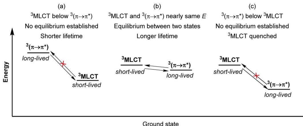
Fig. 17 Simplified qualitative energy level diagrams illustrating the triplet reservoir effect. (a) Typical situation with  $^3\text{MLCT}$  below  $^3(\pi \rightarrow \pi^*)$ . (b) Triplet equilibrium between  $^3\text{MLCT}$  and  $^3(\pi \rightarrow \pi^*)$ . (c) Quenching of  $^3\text{MLCT}$  by lower-energy  $^3(\pi \rightarrow \pi^*)$ .
