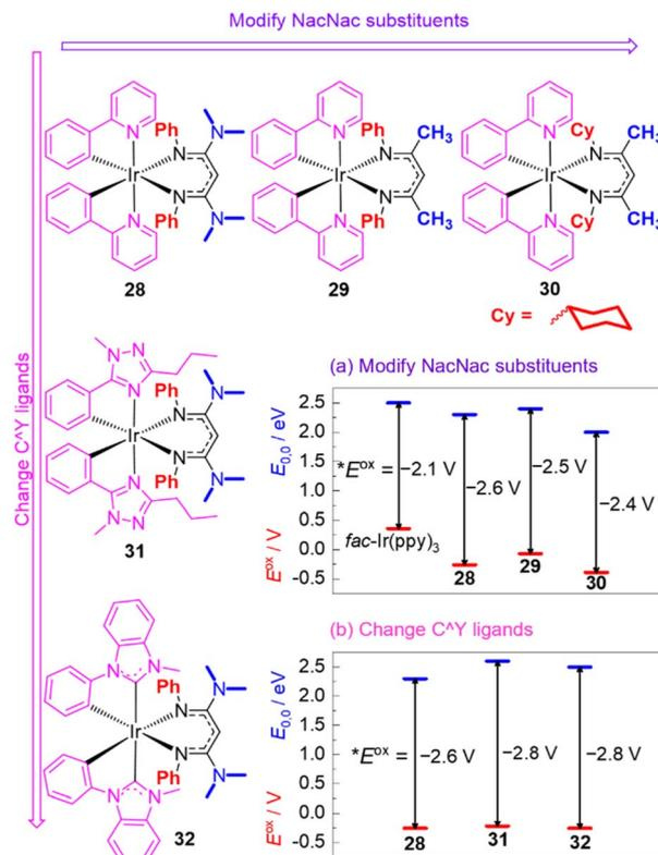
Fig. 12 Summary of representative Ir(C<sup>Y</sup>)<sub>2</sub>(NacNac) photosensitizers, demonstrating structure–property relationships involving  $E^{\text{ox}}$  (red lines) and  $E_{0,0}$  (blue lines). The  $E^{\text{ox}}$  values are referenced to the ferrocene couple, and the vertical arrows represent the absolute value of  $*E^{\text{ox}}$ , as per eqn (1).
