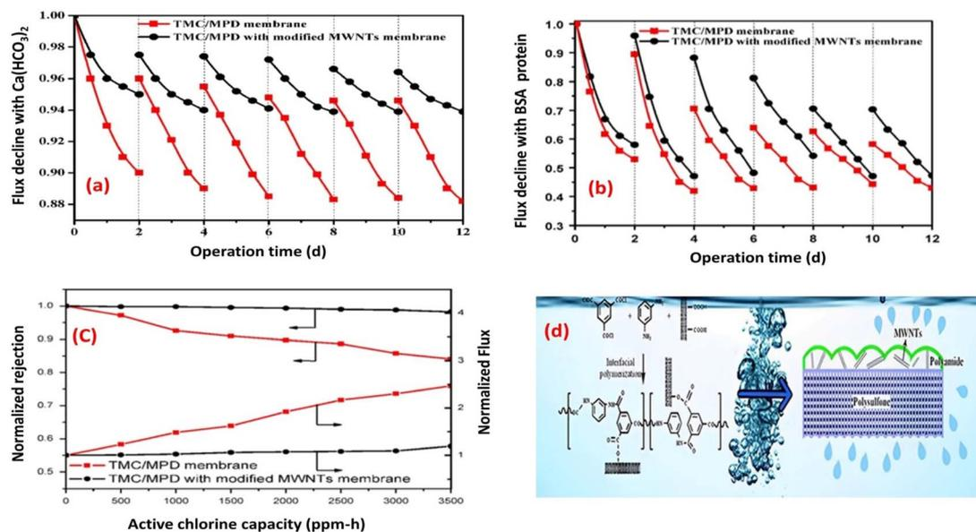
Fig. 7 Flux decline for TMC/MPD and TMC/MPD/MWNTs membranes due to (a)  $\text{Ca}(\text{HCO}_3)_2$ , (b) BSA-protein foulant, (c) RO performance under the active chlorine, and (d) schematic fabrication of TMC/MPD/MWNTs membrane. Reprinted with the permission of ref. 73, copyright 2024, Elsevier.
