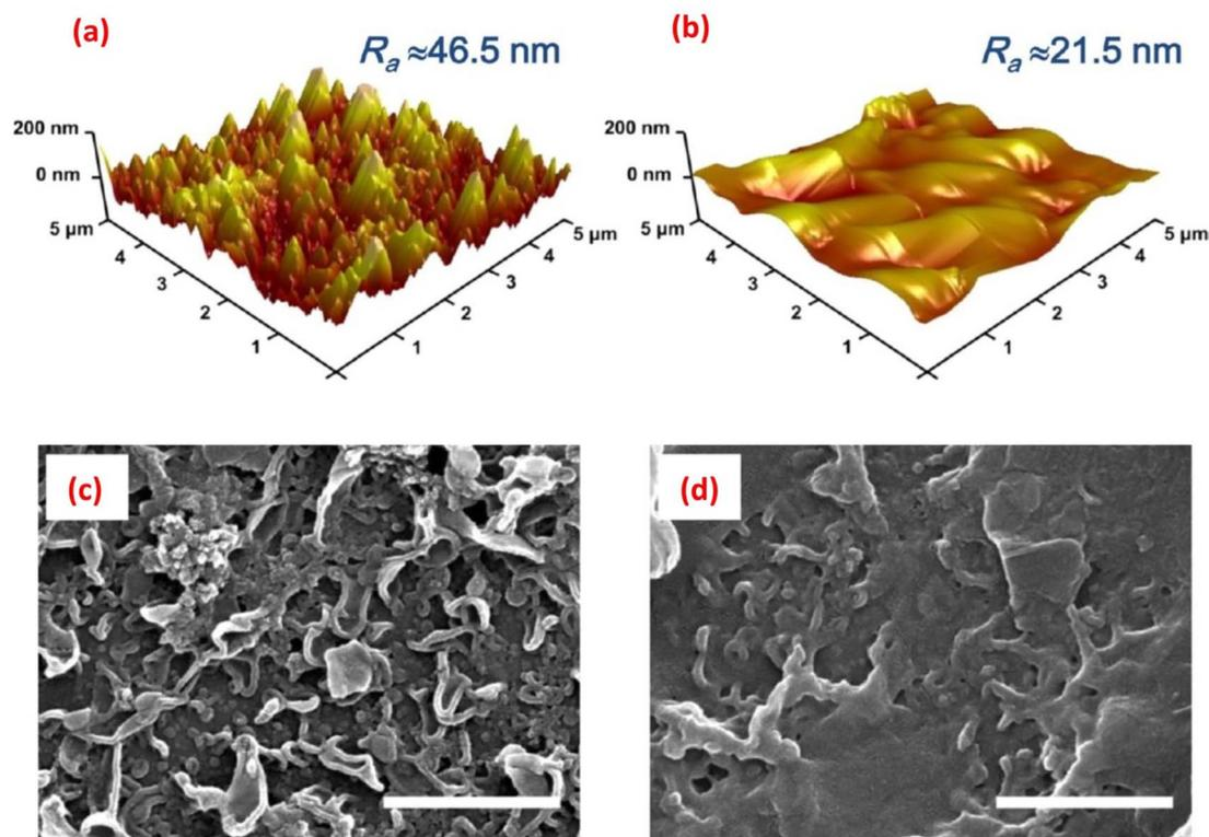
Fig. 14 AFM height images of (a) the pristine, uncoated polyamide (PA) and (b) the GO<sub>10</sub>-coated PA membranes; and the SEM images of (c) the pristine PA and (d) the GO<sub>10</sub>-coated PA membranes, (scale bar = 1 μm). Reprinted with the permission of ref. 29, copyright 2024, American Chemical Society.
