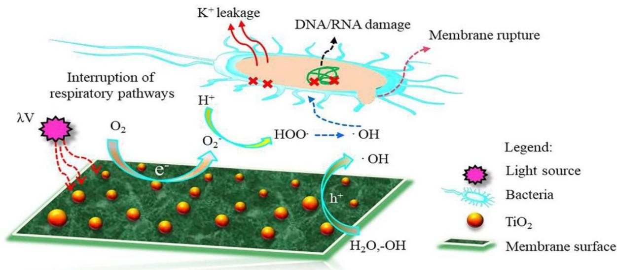
Fig. 10 Proposed mechanism of ROS formation on the surface of TiO<sub>2</sub> NPs-modified TFC membrane. Reprinted with the permission of ref. 135, copyright 2024, Elsevier.
