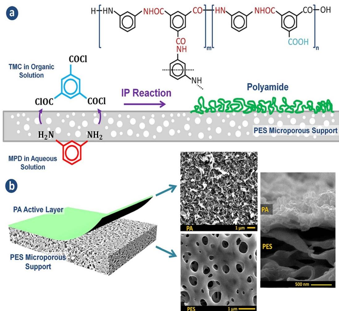
Fig. 1 (a) The interfacial polymerization process between TMC and MPD on a microporous support layer. (b) Structure of the fabricated TFC membranes with the top and cross-sectional morphologies.<sup>148</sup>
