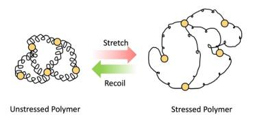
Scheme 3 Elastomer in relaxed state and stressed state in the presence of force
