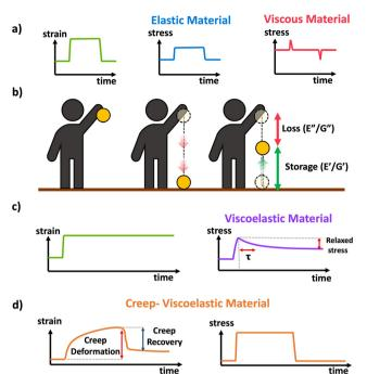
Scheme 11 (a) Schematic of stress response to strain applied to a perfectly elastic (blue) and perfectly viscous (red) material, (b) conceptual demonstration of viscoelasticity in the context of a ball dropped (image inspired by slide 15 from ref. 89), (c) schematic response of a viscoelastic material to applied strain in a stress relaxation experiment. (d) Schematic response of a viscoelastic material to a transiently applied stress in a creep experiment.
