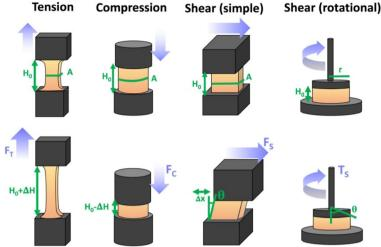
Scheme 9 Typicalmodes of mechanical deformation and testing including tension, compression simple shear and rotational shear. Green arrow shows the direction of the force (F) or torque (T) applied to deform the material, blue highlights the pertinent dimensional parameter. A refers to cross sectional area, r refers to radius,  $H_0$  refers to initial height. Displacements are given as either  $\Delta H$  in tension or compression,  $\Delta x$  in simple shear or  $\theta$  in rotational shear.
