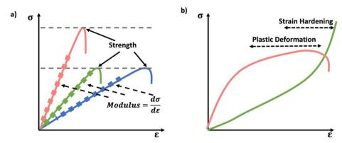
Scheme 10 (a) Schematic stress—strain curves, showing strength as the peak of the stress—strain curve and modulus as slope of stress—strain curve (b) examples of non-linear stress—strain behavior of plastic deformation and strain hardening/stiffening. Plastic deformation leads to a plateau in stress strain properties typically after a yield point, where linearity in the stress strain curve breaks down. Strain hardening manifests a rapid rise of stress with applied strain.
