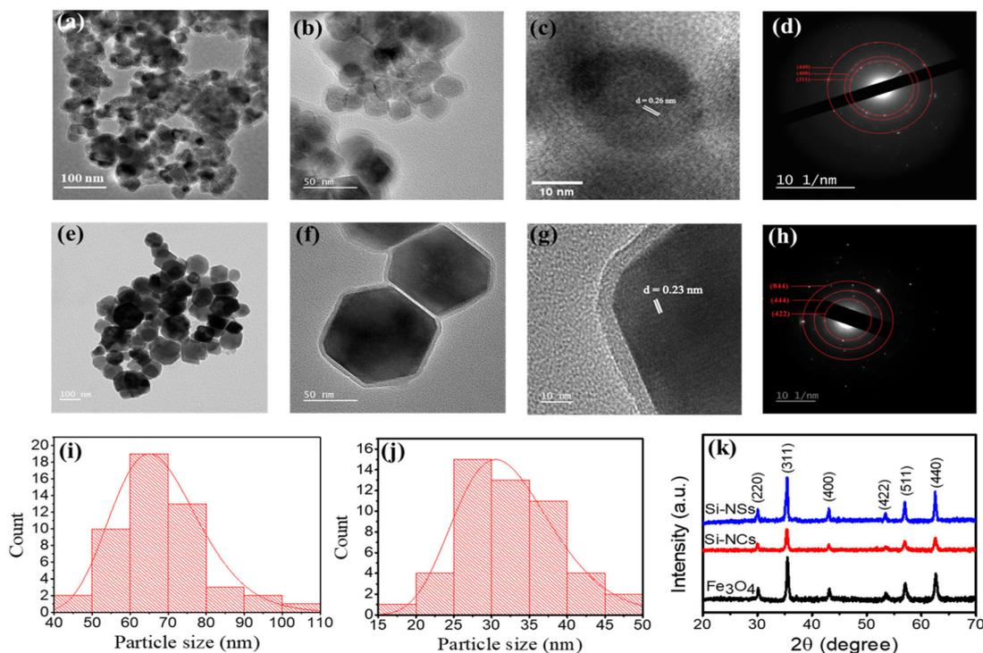
**Fig. 1** Characterization of the synthesised MNPs: (a–c) and (e–g) TEM images of Si-NSs and Si-NCs, respectively, at different scales; (d) and (h) SAED patterns and (i) and (j) size distribution histograms of Si-NSs and Si-NCs, respectively; and (k) XRD patterns of uncoated  $\text{Fe}_3\text{O}_4$  and silica-coated MNPs.
