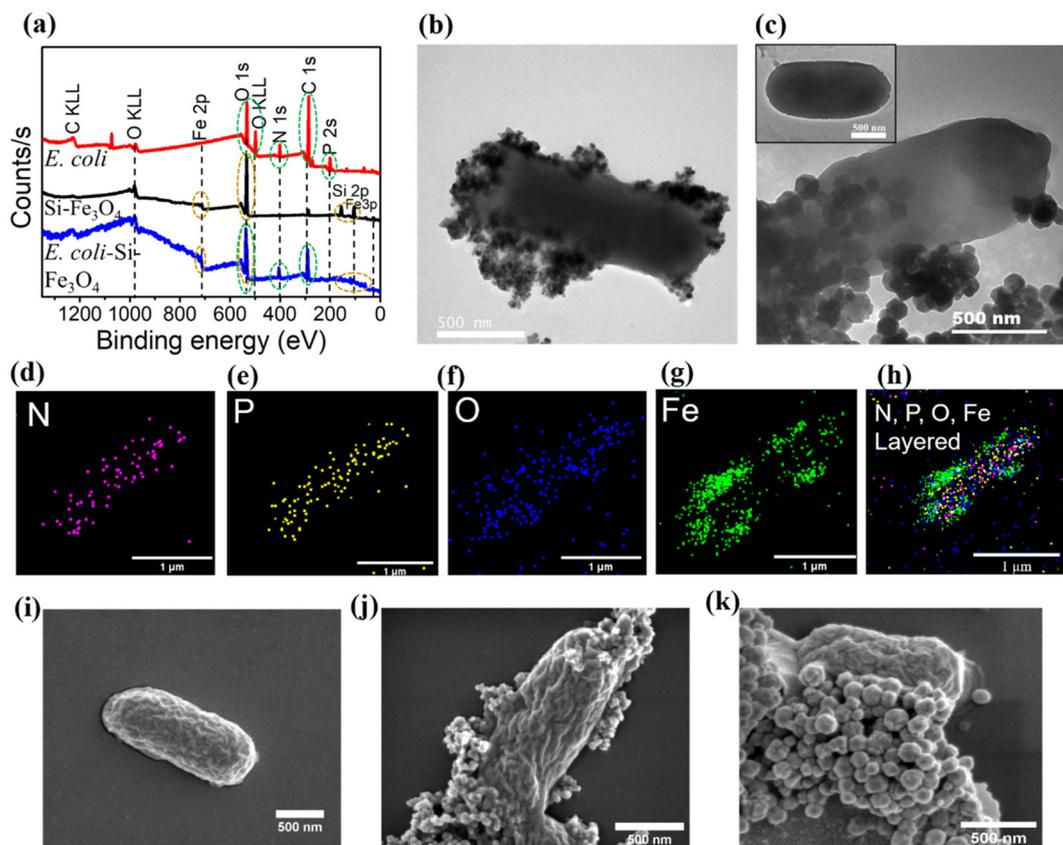
**Fig. 2** Characterization of BacMags: (a) XPS survey spectra of Si-MNPs, *E. coli* and BacMags; (b and c) TEM images of Si-NS-BacMag and Si-NC-BacMag, respectively, where the inset of (c) shows *E. coli* control; elemental mappings of (d) nitrogen, (e) phosphorus, (f) oxygen, (g) iron and (h) merged image of (d–g) of the synthesised BacMags; and SEM images of (i) *E. coli*, (j) Si-NS-BacMag and (k) Si-NC-BacMag.
