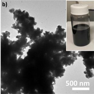
Fig. 1 (a) PXRD of the obtained black  $In_2O_{3-x}$  compared to the simulated pattern for bixbyite  $In_2O_3$ . (b) TEM image of the black  $In_2O_{3-x}$  showing dense agglomerations. The inset shows a picture of the particles dispersed in toluene.
