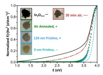
Fig. 4 Kubelka–Munk plot of the black  $\ln_2 O_{3-x}$ , 30 minutes of air flow, air annealed, 120 nm, and 9 nm nanoparticles using  $r=\frac{1}{2}$  for the direct transition. Inset shows dried powders of each of the measured nanoparticles.
