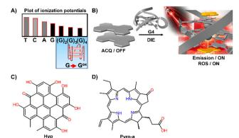
Fig. 9 (A) Plot of ionization potentials showing that guanine has the lowest potential, making quanine-rich sequences particularly susceptible to oxidation. (B) Schematic representation showing how a G4 mediates the disassembly of ACQ-active dyes, restoring their fluorescence properties and facilitating the generation of ROS. (C) and (D) Chemical structures of Hyp and Pyro-a.
