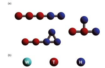
Fig. 1 Particle models used for calculations. (a) Representative modeled amphiphilic molecules composed of two types of DPD beads: hydrophobic tail (red) and hydrophilic head (blue). (b) Coarse-grained DPD beads used in this study. The water bead as solvent (cyan), hydrophobic tail bead (red), and hydrophilic head bead (blue) are labeled W, T, and H, respectively.
