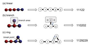
Fig. 2 Modified-SMILES for the linear transformation of coarsegrained molecular models; linear transformation methods for (a) linear, (b) branched, and (c) ring structures.
