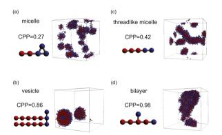
**Fig. 4** Representative snapshots of equilibrium morphologies of amphiphilic molecules and CPPs of their models: (a) micelle, (b) vesicle, (c) threadlike micelle, and (d) bilayer.
